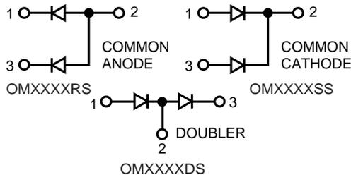
Common cathode is standard. Contact the factory for performance characteristics for common anode and doubler. Z-Tab package also available.
