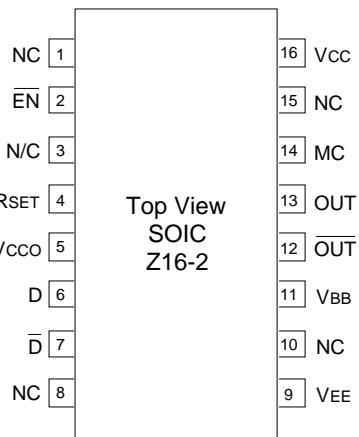
16-Pin Narrow SOIC (Z16-2)
