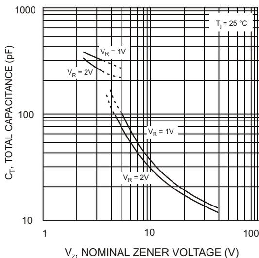
Fig. 4 Total Capacitance vs Nominal Zener Voltage
