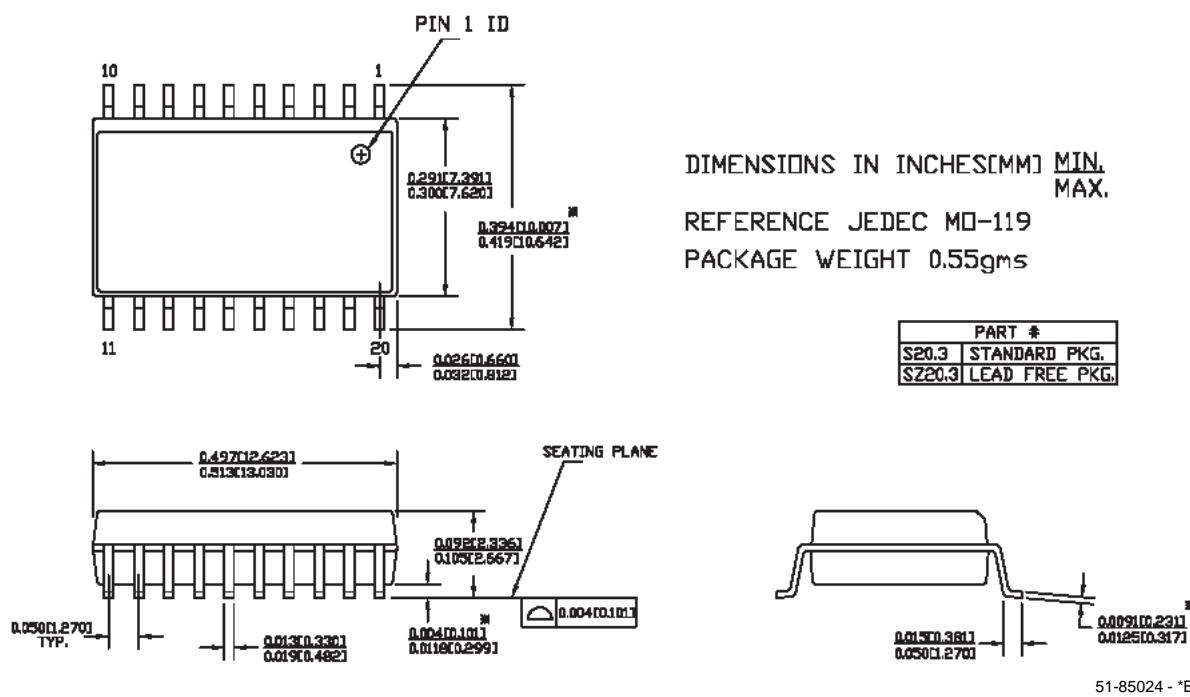
Figure 4-3. 20-Lead (300-Mil) Molded SOIC
