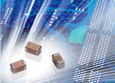
The QM series has been designed to significantly reduce noise characteristics while providing high capacitance values and a low voltage coefficient, making it ideal for mobile phone, hard disk drive, and LCD panel driver circuit application. QM series is based on X5R temperature characteristics with temperature variation of capacitance within +15% from -55°C to +85°C. This capacitance change is non-linear. Capacitance for X5R will also vary under applied voltage and frequency.
