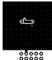
a. 60°C/W when mounted on a 1 in<sup>2</sup> pad of 2 oz copper
