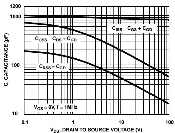
Figure 6. Capacitance vs Drain to Source Voltage
