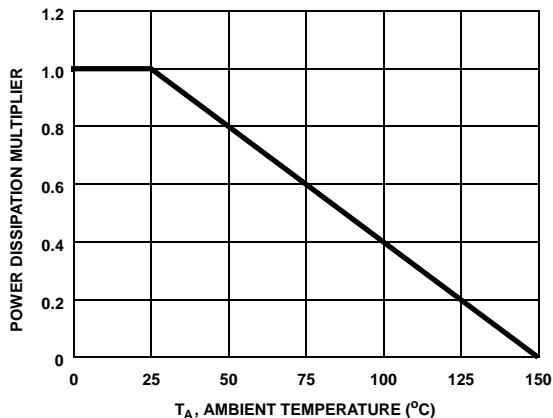
Figure 9. Normalized Power dissipation vs Ambient Temperature
