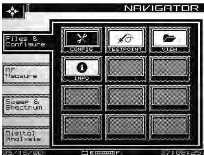
The Navigator user interface, common on all JDSU SDA meters
