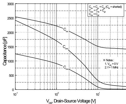
**Figure 5. Capacitance Characteristics**
