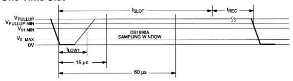
$$60 \ \mu s \le t_{SLOT} < 120 \ \mu s$$
