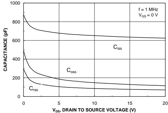
**Figure 8. Capacitance Characteristics.**
