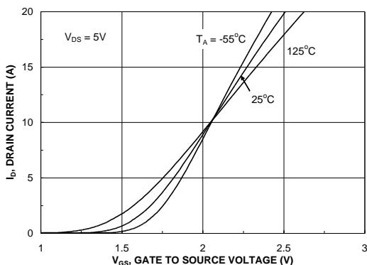
**Figure 5. Transfer Characteristics.**
