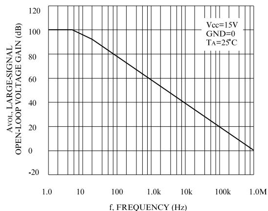
**Figure 2. Open-Loop Frequency**
