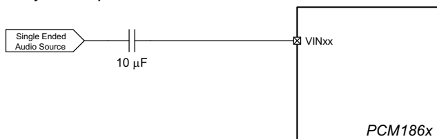
Figure 52. Analog Input Circuit for Single Ended Input Applications
