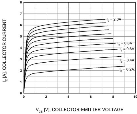
Figure 1. Static Characteristic
