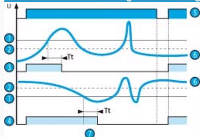
If "with memory" mode has been selected, the relay opens and stays in this position when threshold crossing is detected.
