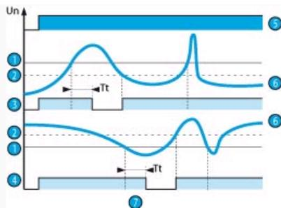
In overvoltage mode, if the controlled voltage exceeds the preset threshold for longer than the time set on the front face (0.1 to 3 s), the output relay opens and LED R is extinguished. During the time delay, this LED flashes.
