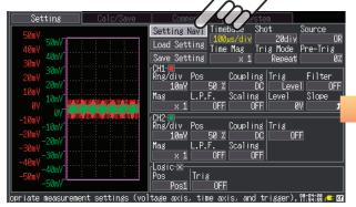
When powered on, the Settings screen appears along with the waveform monitor, and the new Settings Navigator blinks. By activating the Settings Navigator, you can easily navigate by following the simple instructions. Soon you will be operating the device like a seasoned professional.
