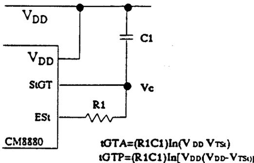
Figure 3. Basic Steering Circuit
