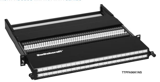
The Front Access Series offers the end user the ease of re-terminating patchpoints from the front of the rack as opposed to the back. A slide out tray allows the user to slide out the punchdown terminals, and reconfigure the unit. An easy release mechanism on either side of the unit allows it to be pushed back into place and easy to grip locking nuts tighten the unit in place.
