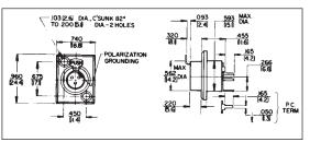
Female receptacle mounts in minimum space from front or rear panel or chassis. Terminals are solder lugs, Series TY(\*)F, or P.C., Series TY(\*)FPC. All receptacles have separate ground lug.
