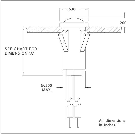
Mounting: Will snap-fit into Ø.500/.505 hole in panels .020/.100 thick. Push-on speednut SN0461 also available.
