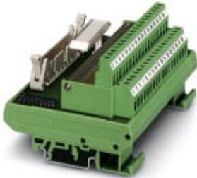
VARIOFACE module, with screw connection and flat-ribbon cable connector, for mounting on NS 32 or NS 35/7.5, with pin strip and short and long locking latches for socket strips, 64-pos., with light indicator
