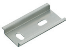
TS 35/7.5 mm according to EN 50022 (s = 1.0 mm)
