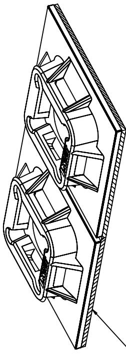
ADHESIVE BACKING: ACRYLIC BASED ADHESIVE, PRESSURE SENSITIVE FOAM TAPE 0.04 (.11.0) THICK WITH A PROTECTIVE LINER. MOUNT IS DESIGNED TO SUPPORT 0.50 lbs (227g) MAX. WEIGHT ON A CLEAN DRY SMOOTH SURFACE.
