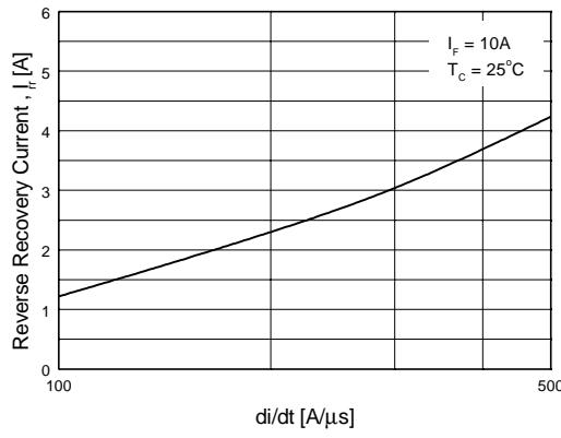
**Figure 5. Typical Reverse Recovery Current vs.  $\frac{di}{dt}$**
