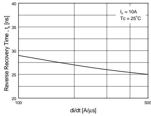
**Figure 4. Typical Reverse Recovery Time vs.  $\frac{di}{dt}$**
