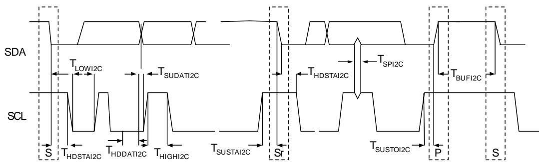
**Figure 3-10. Definition for Timing for Fast/Standard Mode on the I<sup>2</sup>C Bus**
