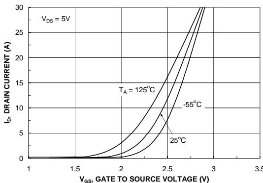
**Figure 5.** Transfer Characteristics.
