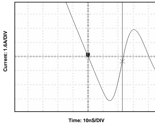
**Figure 24. Non-SyncFET (FDS6982) body diode reverse recovery characteristic.**
