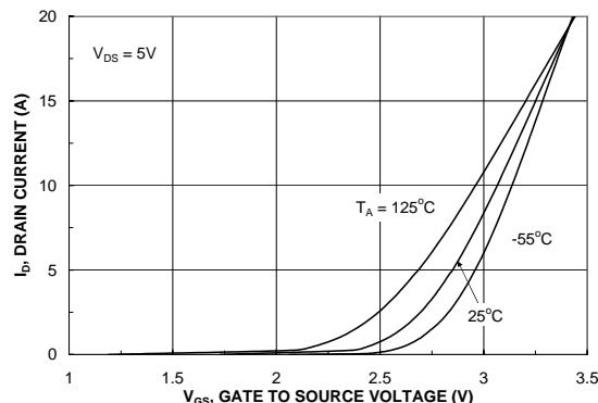
**Figure 16. Transfer Characteristics.**
