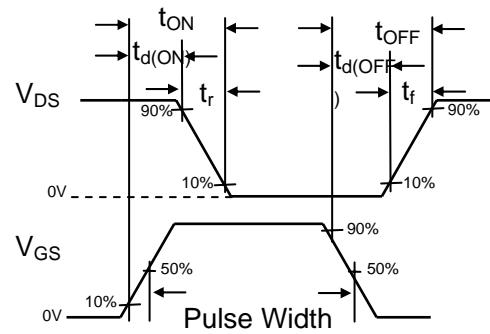
Figure 31. Switching Time Waveforms
