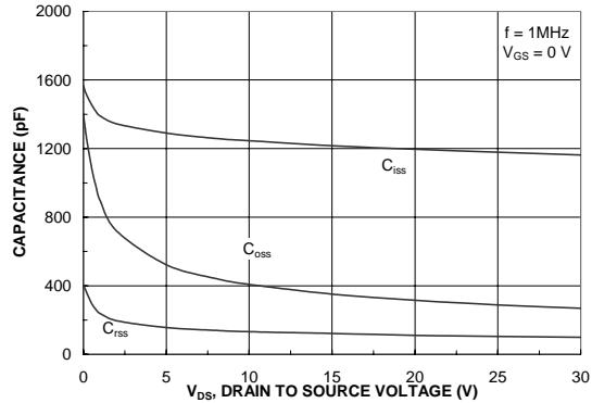
Figure 8. Capacitance Characteristics.
