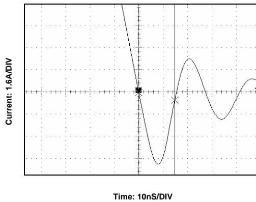
**Figure 23. FDS6982AS SyncFET body diode reverse recovery characteristic.**
