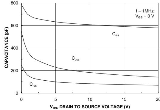
**Figure 19. Capacitance Characteristics.**
