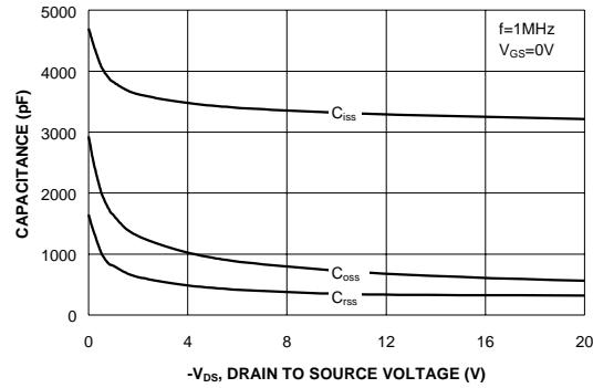
**Figure 8. Capacitance Characteristics.**
