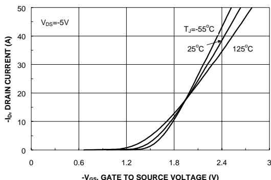
Figure 5. Transfer Characteristics.
