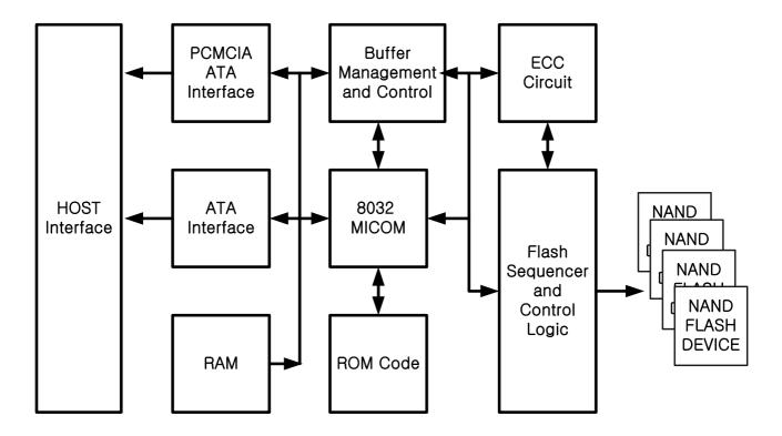
Figure 2.1 Block Diagram
