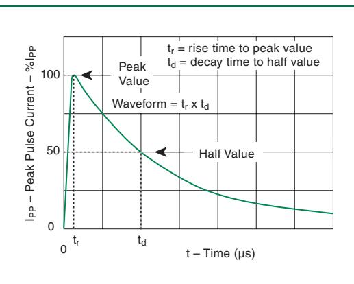
**t<sub>r</sub> x t<sub>d</sub> Pulse Waveform**
