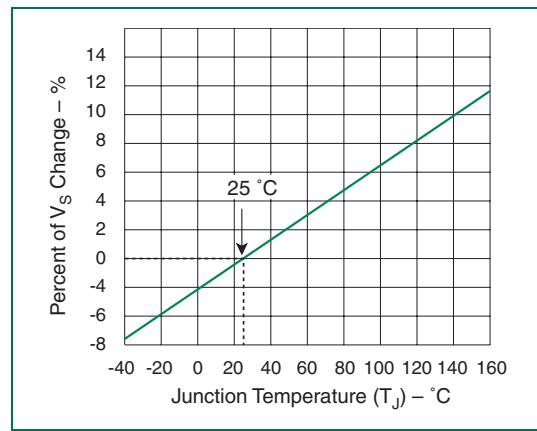
**Normalized V<sub>S</sub> Change versus Junction Temperature**
