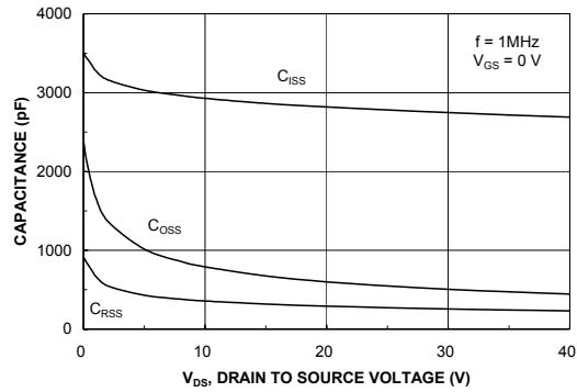
**Figure 8. Capacitance Characteristics.**
