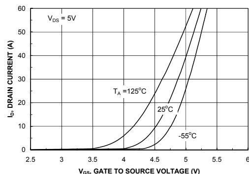
**Figure 5. Transfer Characteristics.**
