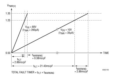
Figure 2. Overcurrent Fault Timer Current
