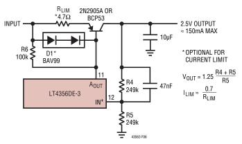
Figure 6. Auxiliary LDO Output with Optional Current Limit
