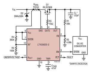
Figure 9. Overvoltage Regulator with Low-Battery Detection
