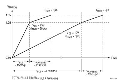
Figure 1. Overvoltage Fault Timer Current
