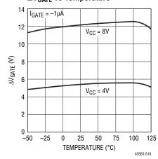
$\Delta V_{GATE}$  vs  $V_{CC}$
