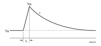
Figure 3. Prototypical Transient Waveform
