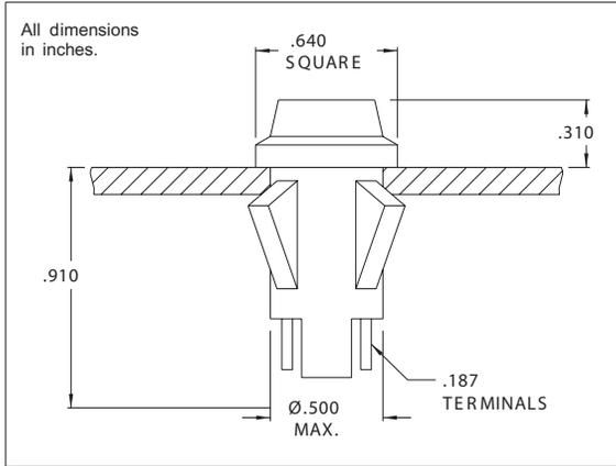
Mounting: Will snap-fit into  $\text{Ø}.500/.505$  hole in panels  $.020/.100$  thick. Push-on speednut SN0461 also available.
