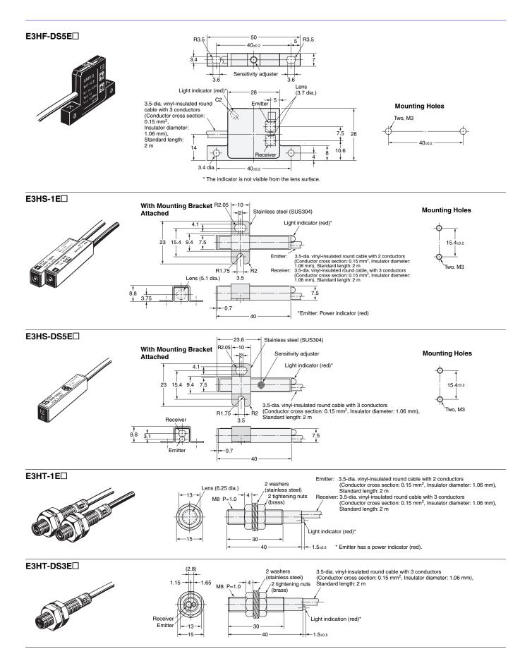
Note: Models numbers for Through-beam Sensors (E3H□-1E□) are for sets that include both the Emitter and Receiver.
