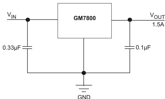
For a positive regulator, a 0.33µF bypass capacitor should be used on the input terminals. While not necessary for stability, an output capacitor of 0.1µF may be used to improve the transient response of the regulator. These capacitors should be on or as near as possible to the regulator terminals .
