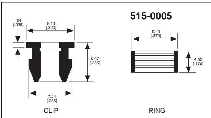
515-0005 Snap-In Mounting Clips for use with the following LEDs:
